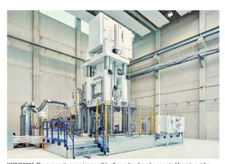
WKP 25000 S: The composite press is accessible all round and can be operated from two sides (© TU Chemnitz)
