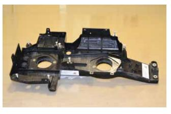
Engine mount of glass-mat-reinforced thermoplastic in combination with thermo-prepreg, which can be manufactured at the IST, thanks to the rapid pressure build-up in the press
